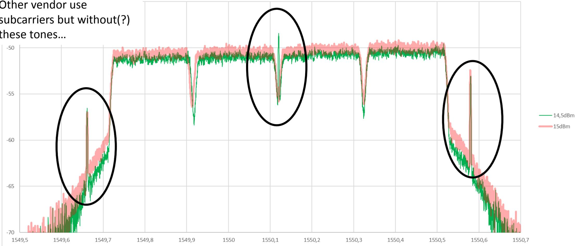
SPM and 300G: 14.5 dBm is the limit for error free transmission.
