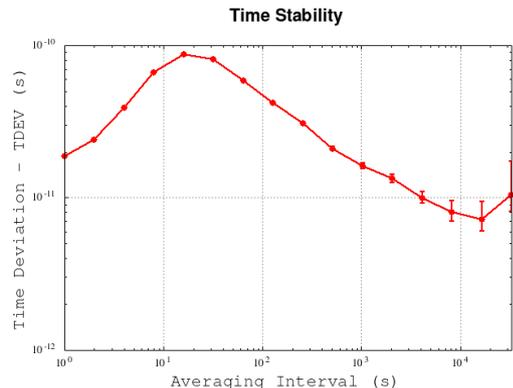
TDEV comparison for TTA and WR transfers over 180 km of field deployed fibre
