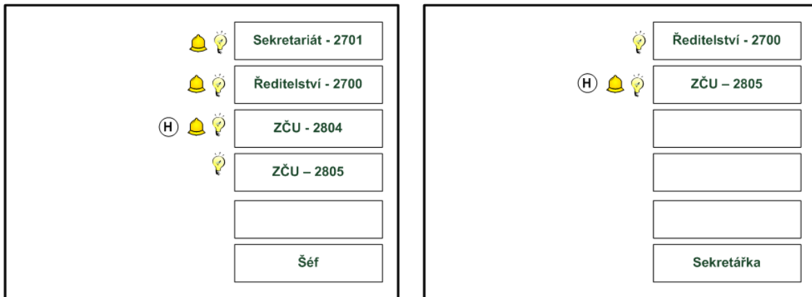
Figure 2. Lines in a Type A setup – assistant’s phone on the left, manager’s phone on the right
